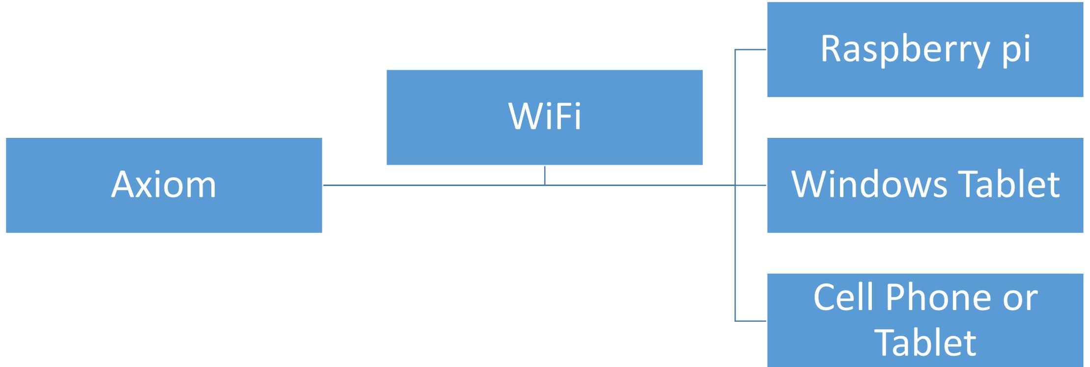
Axiom can log into the internet when available and share its connection with all the other devices. Even without the internet it allows the devices to share data. The Raspberry pi puts data on a web page which can be viewed anywhere on the boat and allows control of anchor light and navigation lights from any device on the network. Pi also runs Signal K
